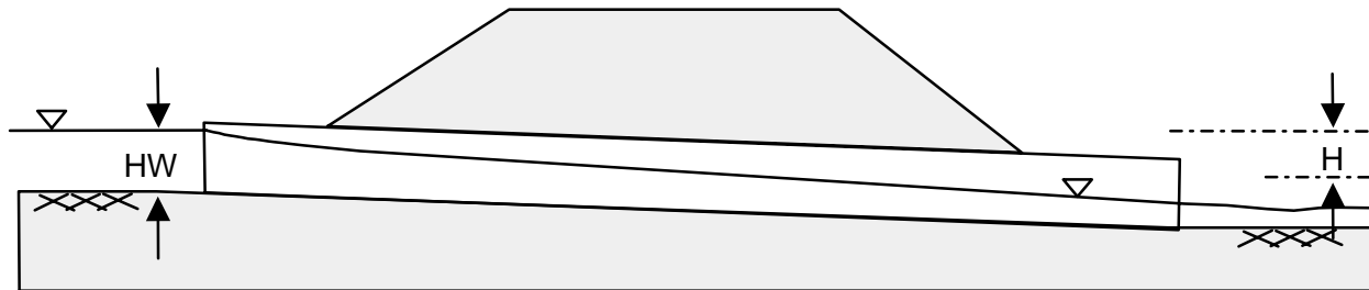
d. Culvert Not Flowing Full
